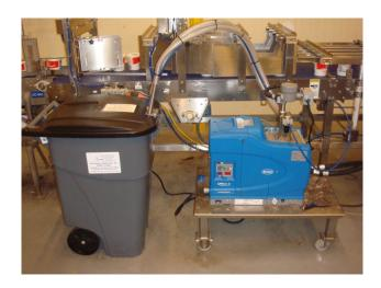
The Northwest Adhesives, Inc. automatic pellet loading system will fit most commercial hotmelt adhesive melters and provide these important benefits.......
